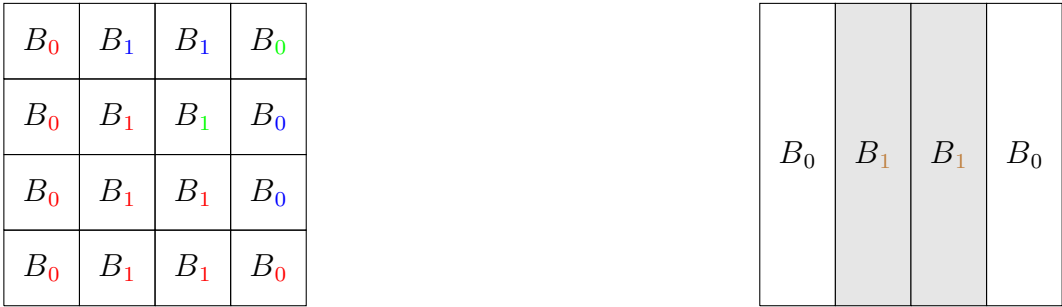
Figure 2: 1D block cyclic partitioning schemes for \text{CH}_4 . Left: the process grid for ERI generation, where submatrices of ERI as in (2) are assigned to two processes. The numbers represent the process the block belongs to. The red font indicates that the block is generated, the green font indicates that the block is also on the same process and can be discovered through transpose, and the blue font indicates that the block is obtained from communication. Right: the process grid for CG solver, where block columns are assigned to the two processes to enable multiplication (8).
